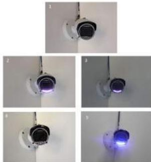
Figure 14. The transmitting surveillance camera, as it seen by a human observer (1) and different camera receivers (2-5).
