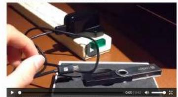
As you can tell from the video above, it is trivial to perform a supply chain attack that modifies the firmware recovery seed. Since all private keys are derived from the recovery seed, the attacker could steal any funds loaded onto the device.
